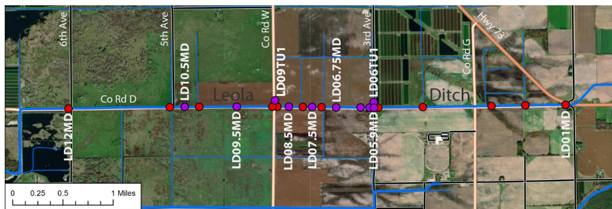
Figure 12. Overview map with satellite imagery over hillshade from 5ft LIDAR data for section of Leola Ditch monitored during this study. Thick blue lines mark larger drainages, thin blue lines represent small tributary ditches. Red circles are surface water sampling stations, purple circles are stations with mini-piezometer installations.
